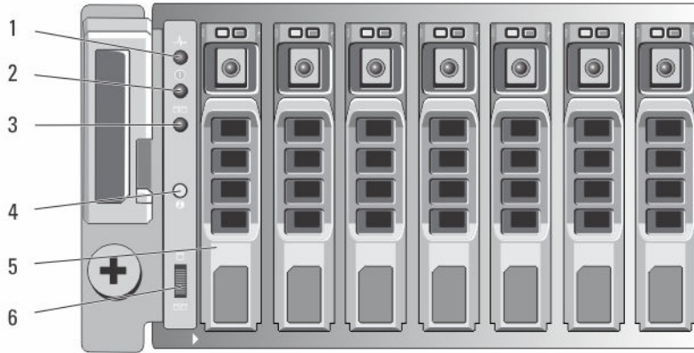
Figure 2. Front-Panel Features and Indicators—Dell PowerVault MD3820f
